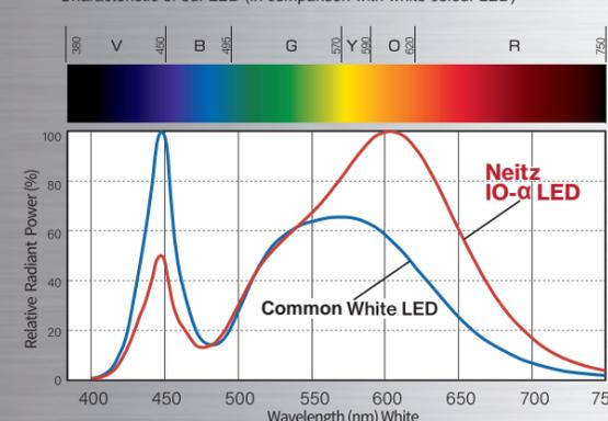
The colour temperature of the LED of Neitz IO-α LED is 3200°K, which is same colour temperature to the halogen bulb used in the typical binocular indirect ophthalmoscope.
